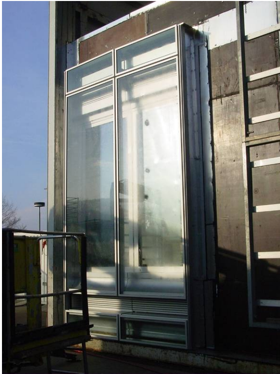
Fig. 1 Facade mounted in test rig
