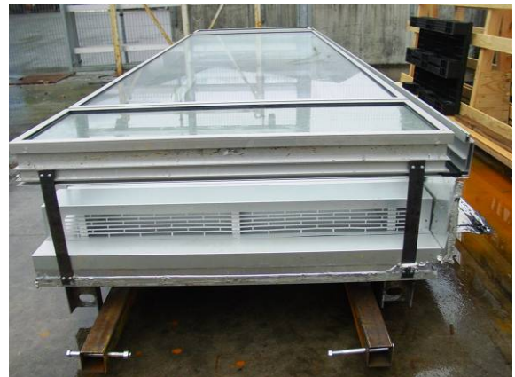
Fig. 30 Dismantled facade unit
