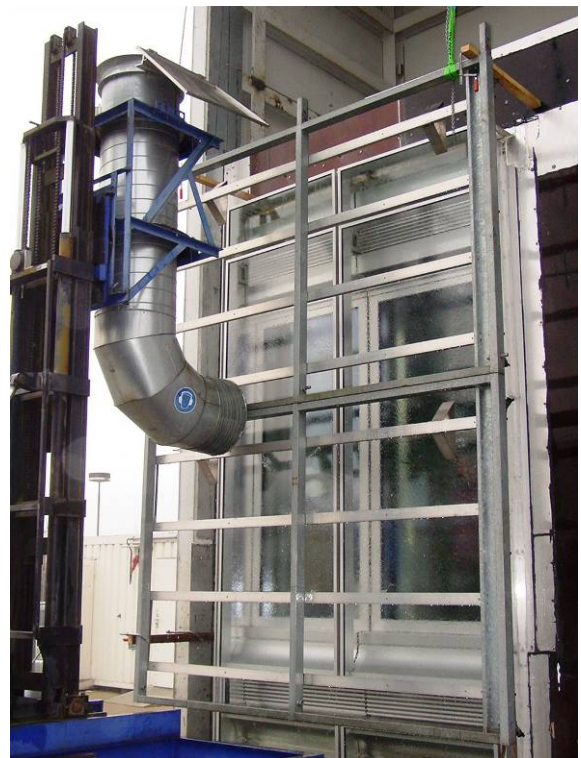
Fig. 4 Dynamic watertightness test
