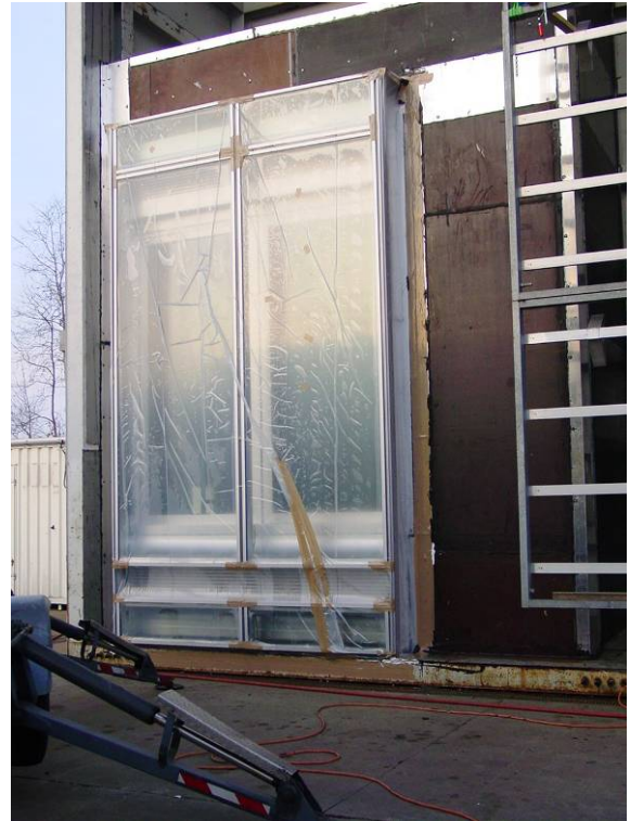
Fig. 2 Façade with film suspended in front for zero measurement
